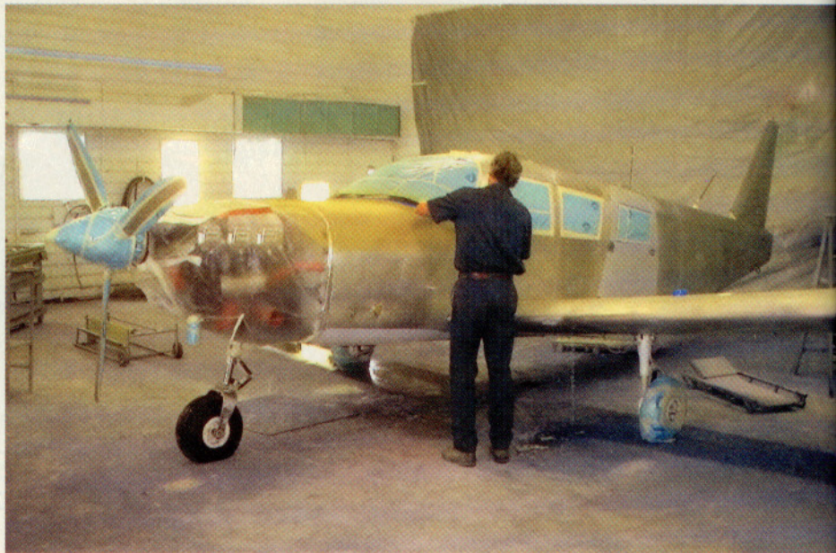
After chemical stripping, surface irregularities are repaired and spot-primed. Here the windows and other critical components are masked off in preparation for a coat of primer. Alodining has turned the aluminum skins a gold color.
